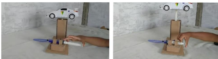
Figure 5. Application of Pascal's Law on Hydrolic Lifts
